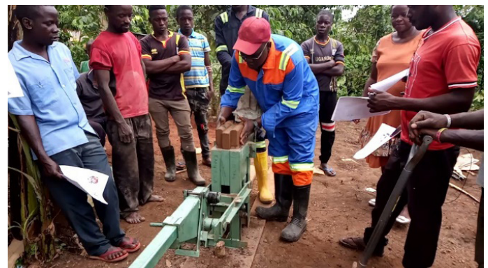
Figure 3: constructing the FEC (left: producing the first environmentally friendly block: Right; constructing FEC)
